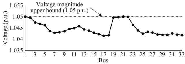
Fig. 8. The voltage profile after applying curtailment.
