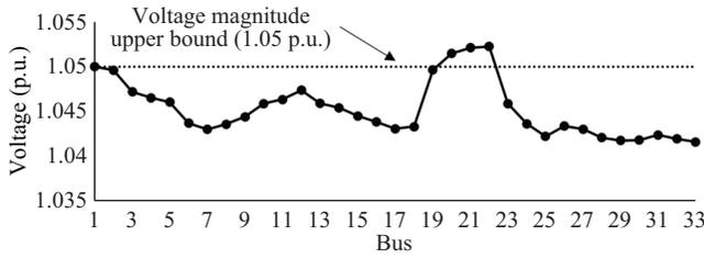
Fig. 7. The voltage profile if no transactions are curtailed.
