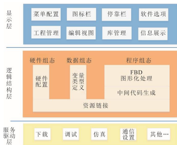
图 4 逻辑组态软件层次化架构 Fig.4 Hierarchical architecture diagram of the logic configuration software
