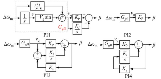
Fig. 4. Transfer function of the PI limiters.
