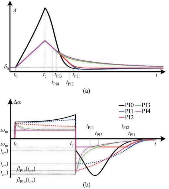
Fig. 9. PI0~PI6 dynamics in the scenario of no equilibrium point. (a) Frequency response. (b) Phase response.
