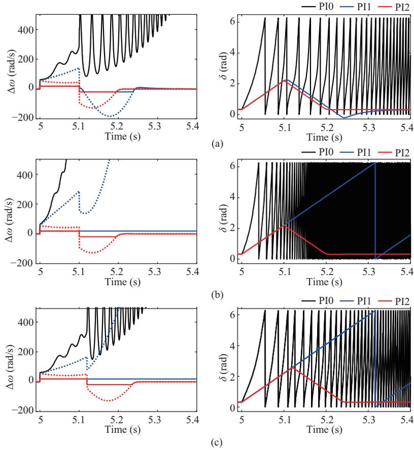
Fig. 13. Comparison of PI1~PI3 in Scenario 2 with different  $K_i$  and  $t_c$ . (a)  $K_i = 0.58$ ,  $t_c = 0.1$  s. (b)  $K_i = 1.18$ ,  $t_c = 0.1$  s. (c)  $K_i = 0.58$ ,  $t_c = 0.12$  s.
