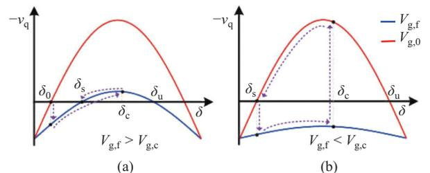
Fig. 5. Classification of the synchronization stability with the fault scenarios. (a) Equilibrium Point exists. (b) Equilibrium point does not exist.
