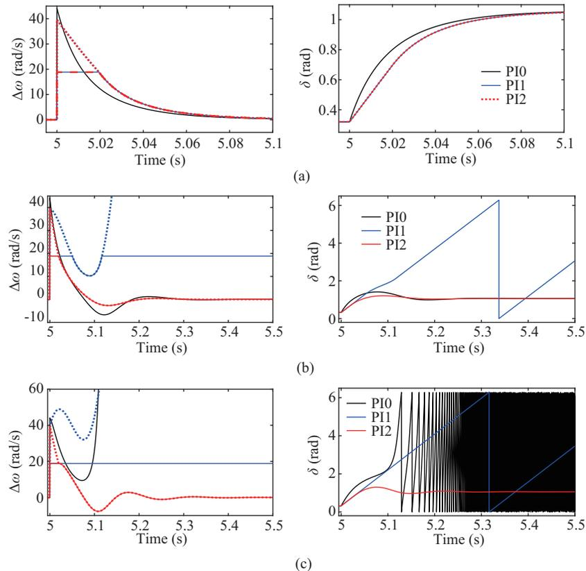
Fig. 10. PI0~PI2 comparison in Scenario 1 with  $K_i$  increasing. (a)  $K_i = 0$ . (b)  $K_i = 0.58$ . (c)  $K_i = 1.18$ .
