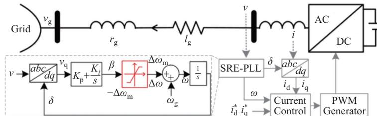
Fig. 1. Structure of a grid-following converter.
