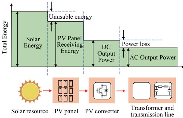
Fig. 1. Overall energy flow of PV generation.
