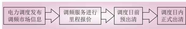
图 4 广东调频市场交易流程 Fig. 4 Guangdong frequency modulation market trading process
