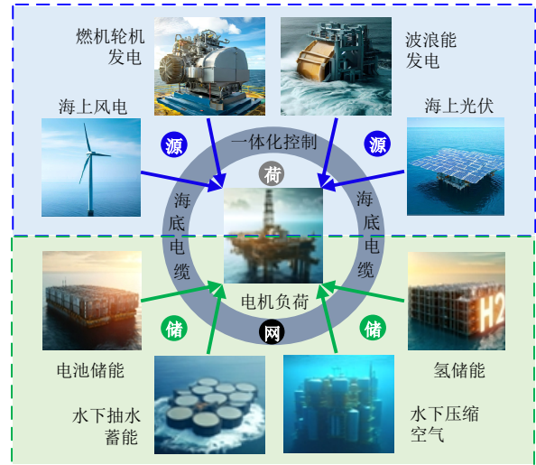
图 2 海上油田群新型电力系统结构 Fig. 2 Structure of new-type offshore oilfield power systems
