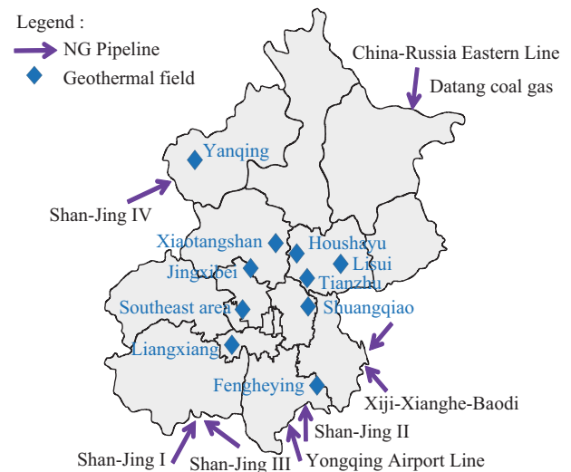
Fig. 7. The natural gas transmission pipelines and main geothermal field distribution of Beijing.
