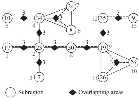
Fig. 12. IEEE 123-bus border-node overlapping equivalent graph constructed for subregion merging.
