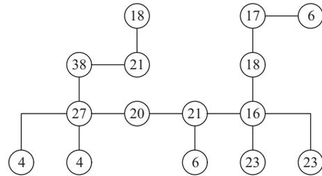
Fig. 6. IEEE 123-bus non-overlapping equivalent graph constructed for subregion merging.
