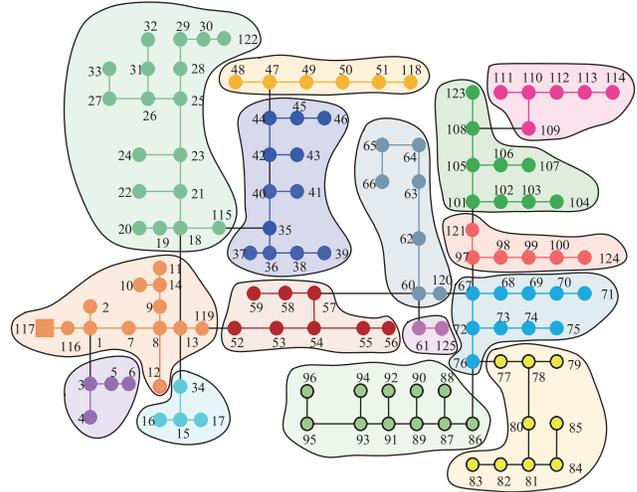
Fig. 5. IEEE 123-bus non-overlapping initial partition result based on community detection.
