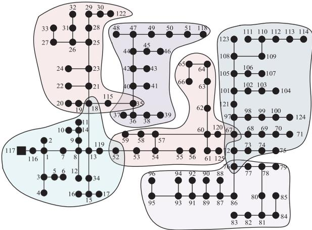
Fig. 13. IEEE 123-bus border-node overlapping partition ( $N = 6$ ).
