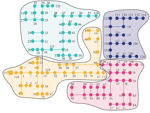
Fig. 9. IEEE 123-bus over-overlapping partition result in [13].
