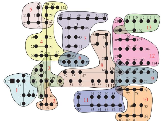
Fig. 11. IEEE 123-bus over-overlapping initial partition result based on community detection.
