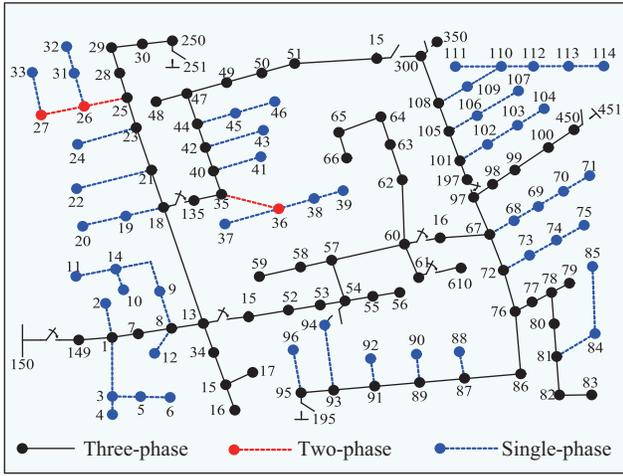
Fig. 3. IEEE 123-bus power system mode.
