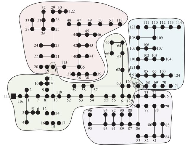
Fig. 15. IEEE 123-bus border-node overlapping partition ( $N = 4$ ) in other literatures.
