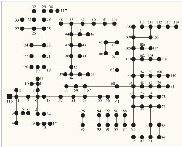
Fig. 4. IEEE 123-bus equivalent weighted undirected topology.
