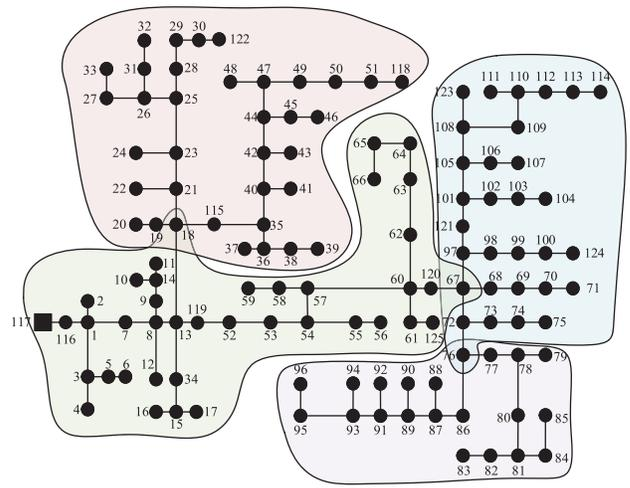
Fig. 14. IEEE 123-bus border-node overlapping partition ( $N = 4$ ).
